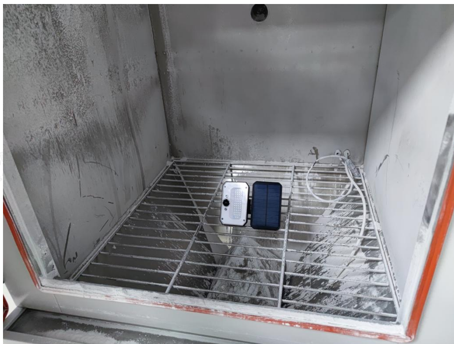
Photo 3: IP5X test of model S5-1600LM
