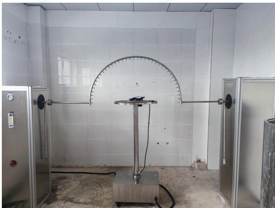
Photo 4: IPX4 test of model S5-1600LM
