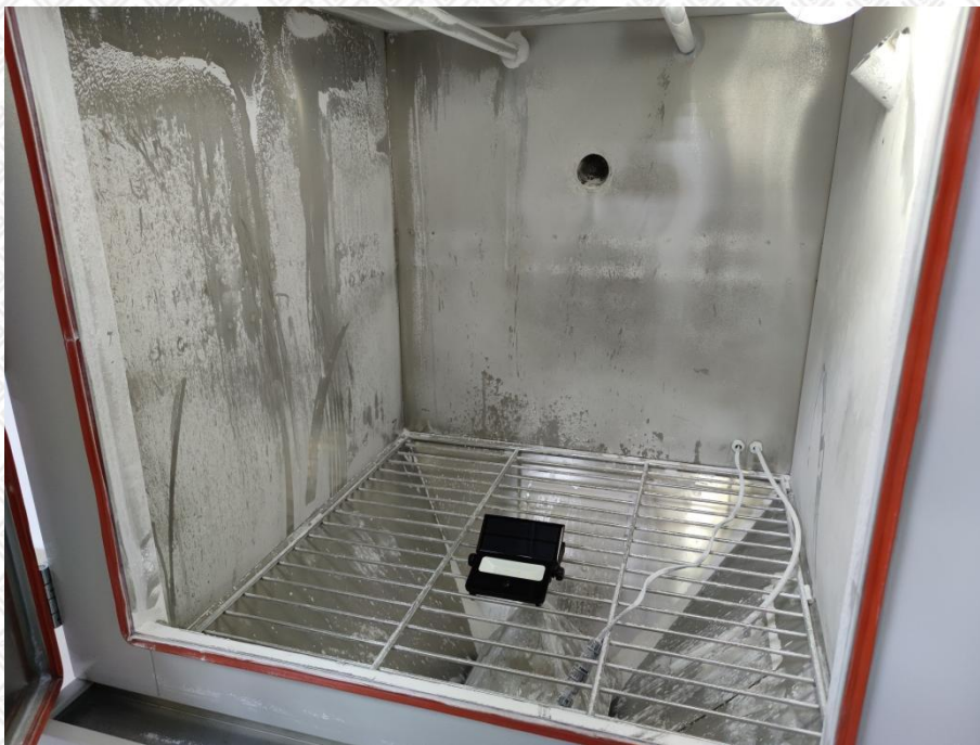
Photo 3: IP5X test of model AL-S3 PIR
