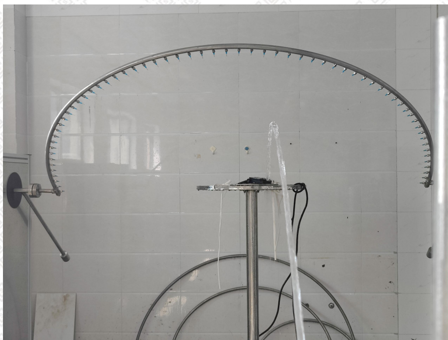
Photo 2: IPX5 test of model AL-S3 PIR
